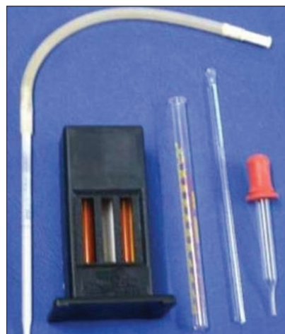
Figure 1: Sahli's Hemoglobinometer with pipette, hemometer tube, stirring rod, and dropper
